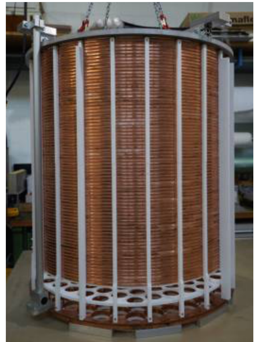
TPC assembly, cool down tests
