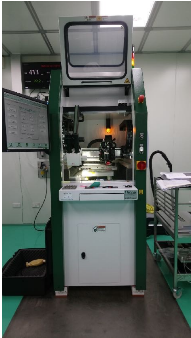
Bonding machine Wire bond
