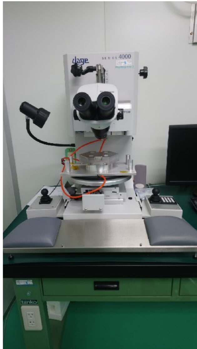
Bondtester Bonding wire quality test
