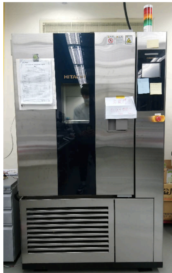
Temperature & humidity chamber Half-ladder/Ladder thermal cycle
