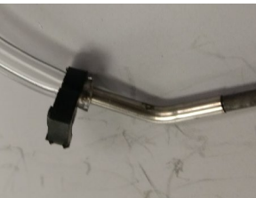
Tygon connected directly to SS tube and clamped (0.25" OD 1/8" ID)
