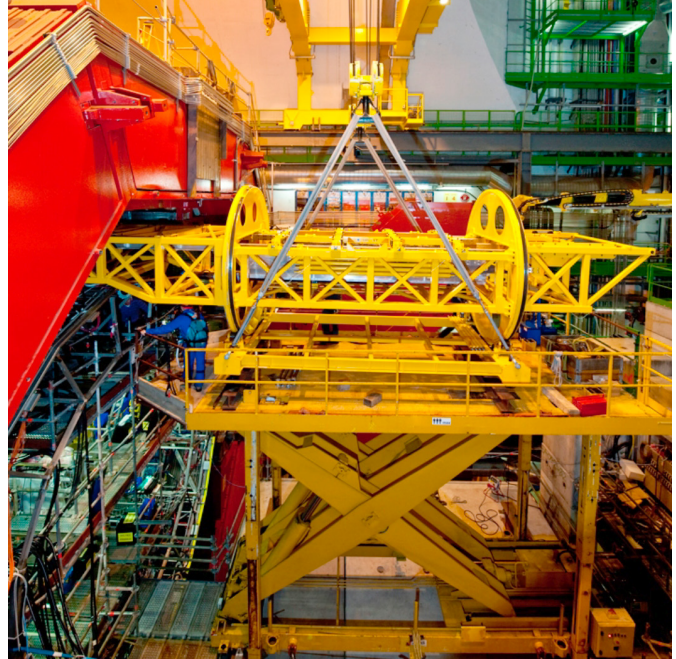
Figure 7.3: View of US-led ALICE ElectroMagnetic Calorimeter (EMCal) modules during installation in the ALICE experiment; one of the 10 EMCal modules, weighing over 7 tons, is being inserted.
