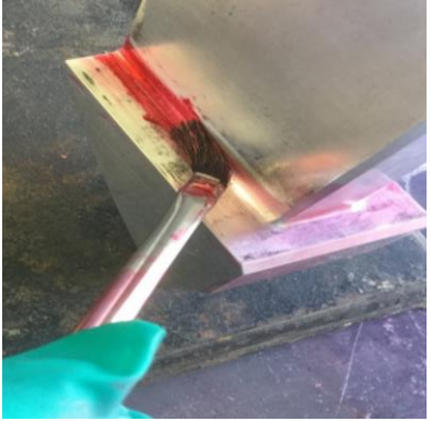
Al clamp test with die penetration technique
