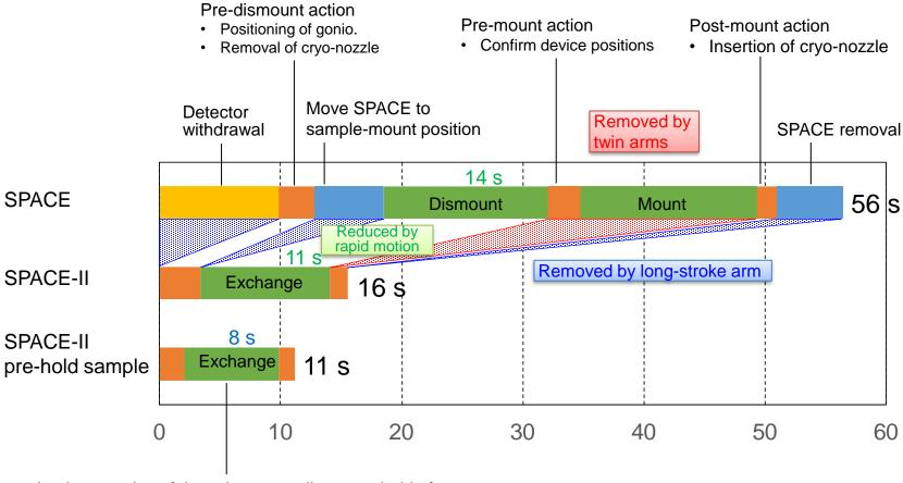
Implementation of the twins arms allows pre-hold of a new sample in the case of automatic data collection.
