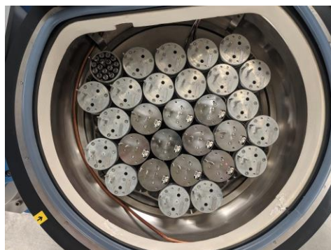
Sample changer dewar with capacity for 464 samples
