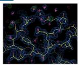
Proteinase K structure refined to 2.0 Å resolution  $\underline{R}_{work}$ =16.7% and  $\underline{R}_{free}$ =21.3% (500Hz dataset)
