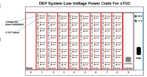
6 1/2 U size crate Same as DEP32 ADC but w/ different PSU mounting plate 8x Power card slots Isolated Common "Floating Ground" 8u Card Width (1.6") 1x Crate controller card CRATE PSU 120/208 VAC to 48VDC 1.4kW
