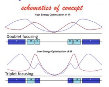
change polarity of quads DDF to FDF
