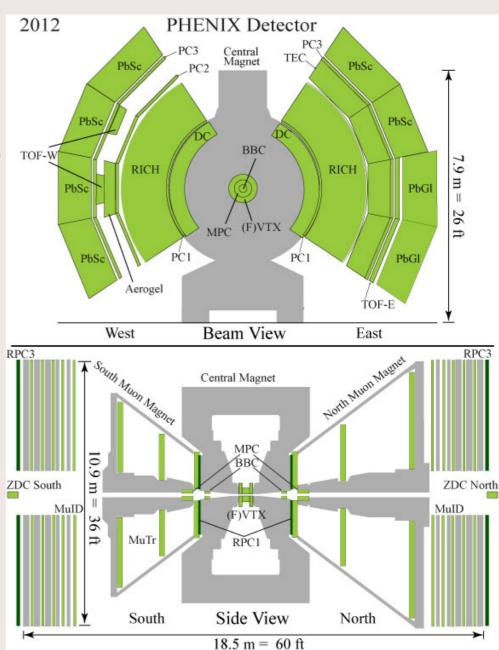
**PHENIX**:  $h, e^{\pm}, \gamma$  in  $|\eta| < 0.35, \phi \in 2 \times \pi/2$ ;  $\mu$  in  $1.2 < |\eta| < 2.2$
