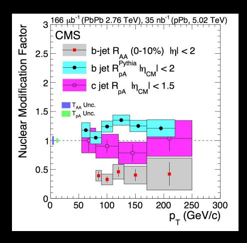
Suppression of b quarks in PbPb, while no apparent suppression in pPb collisions
