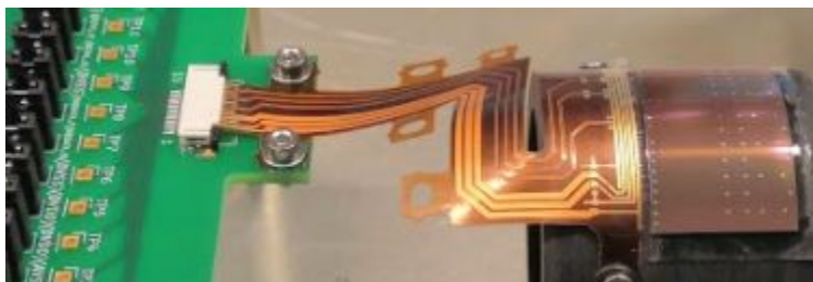
Bent ALPIDE, wire-bonded to bendable FPC, connected to interface card
