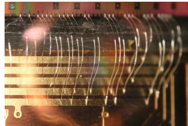
Bent ALPIDE, wire-bonded
