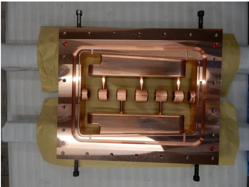
IH-DTL test cavity
