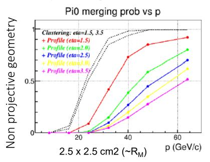
Projective geometry => improved separation, particularly for  $\eta^{\sim}$  1-3
