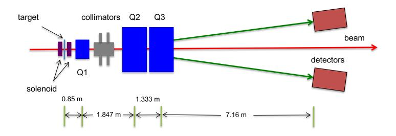
Hall C Møller Polarimeter uses "2-quadrupole" spectrometer that allows fixed optics/acceptance for full energy range
