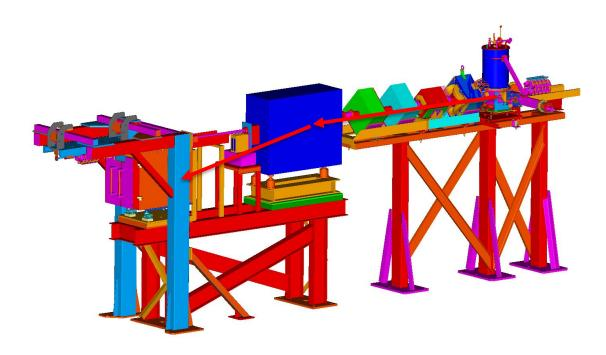
Hall A Møller Polarimeter uses 4-quadrupole + dipole system
