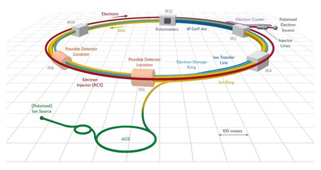
Electrons must be accelerated to full beam energy before entering the electron storage ring
