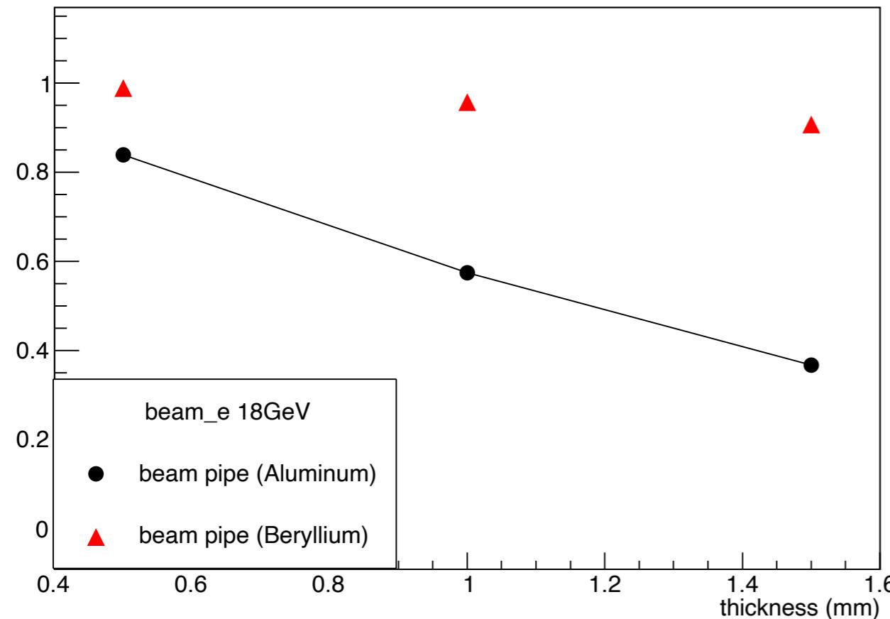
The exit window is not necessary if we can use Beryllium 05mm thickness (~98% acceptance) beam pipe.
