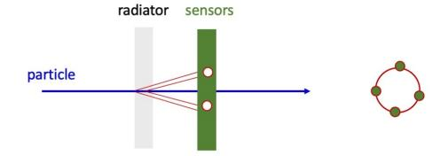
DIRC: photons still need to survive the total internal reflection limit
