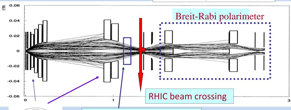
RF transition, polarization transfer from electrons to protons
