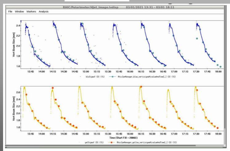
Vertical beam size measurements from IPMs compared with H-jet measurements. From LEReC ELog of 03/01/21:
