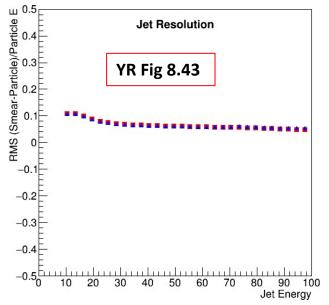
For the YR the JES was calculated as the mean of the smeared jet energy minus the true jet energy divided by the true jet energy
