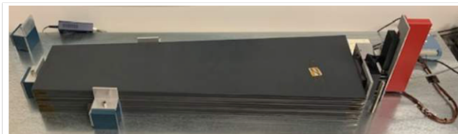
Figure 2.4: Testing the HCal scintillator tiles at GSU.
