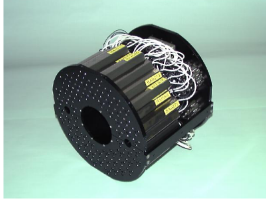
Figure 2.5: The minimum bias detector, originally built by Hiroshima University for PHENIX.
