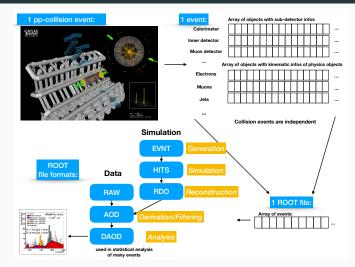
In essence: several steps of data processing and then **data reduction** First parts on Grid/Cloud/HPC - last step usually on local resources
