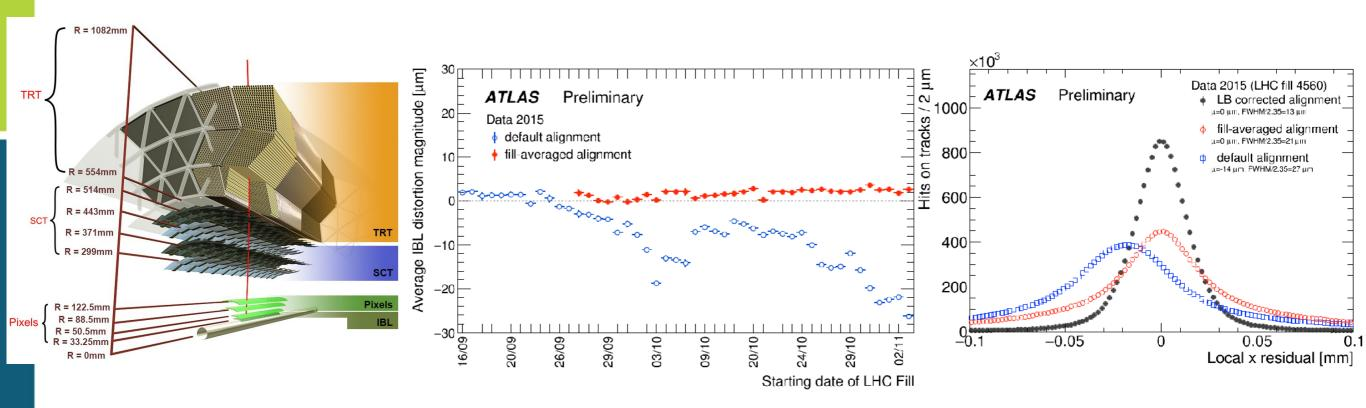
During the break between Run 1 and Run 2, ATLAS inserted the IBL, an extra layer of silicon tracker close to the beam pipe
