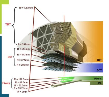
During the break between Run 1 and Run 2, ATLAS inserted the IBL, an extra layer of silicon tracker close to the beam pipe
