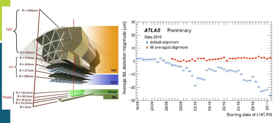
During the break between Run 1 and Run 2, ATLAS inserted the IBL, an extra layer of silicon tracker close to the beam pipe
