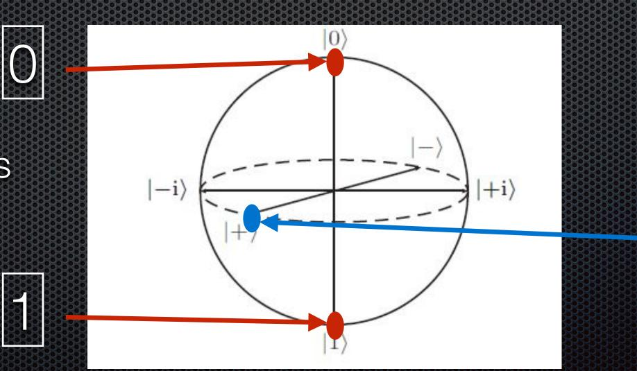
quantum mechanically, any point on the sphere is allowed, e.g. here ("any superposition of 1 and 0")
