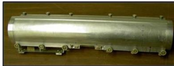
NMR trolley maps the field at about 9000 locations over the entire azimuth every 3 days
