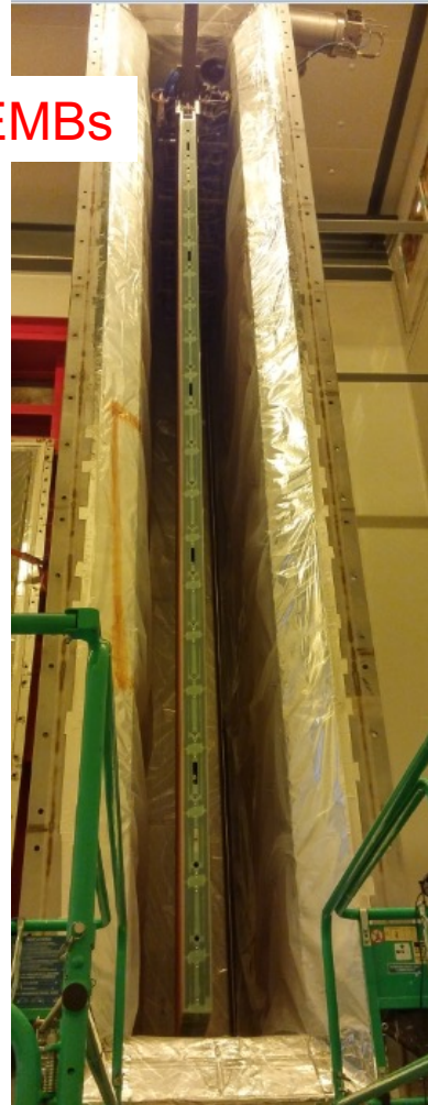
ProtoDUNE APA1 installed in the Cold Box
