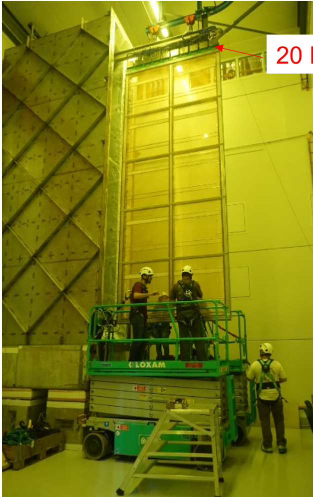
ProtoDUNE APA1 installed in the Cold Box
