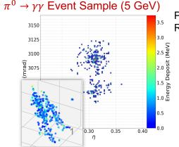
Pixel Readout 0.5×0.5 mm²; 20 ~ 700 keV Dynamic Range; 5 keV Noise Level; 2% Flat Resolution
