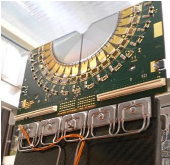
Fig. 1: VELO module with a half-circular silicon sensor, 16 Beetle readout chips, five cooling blocks and the capillaries for the CO 2 supply.
