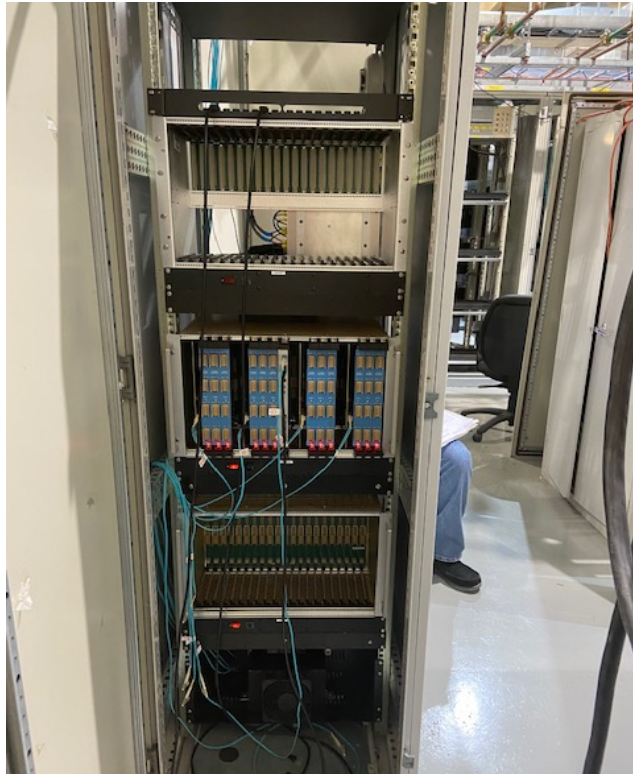
Figure 11: First HCal Digitizer and control rack partially assembled in 1008. Once all modules are installed it will be tested and installed onto the detector.
