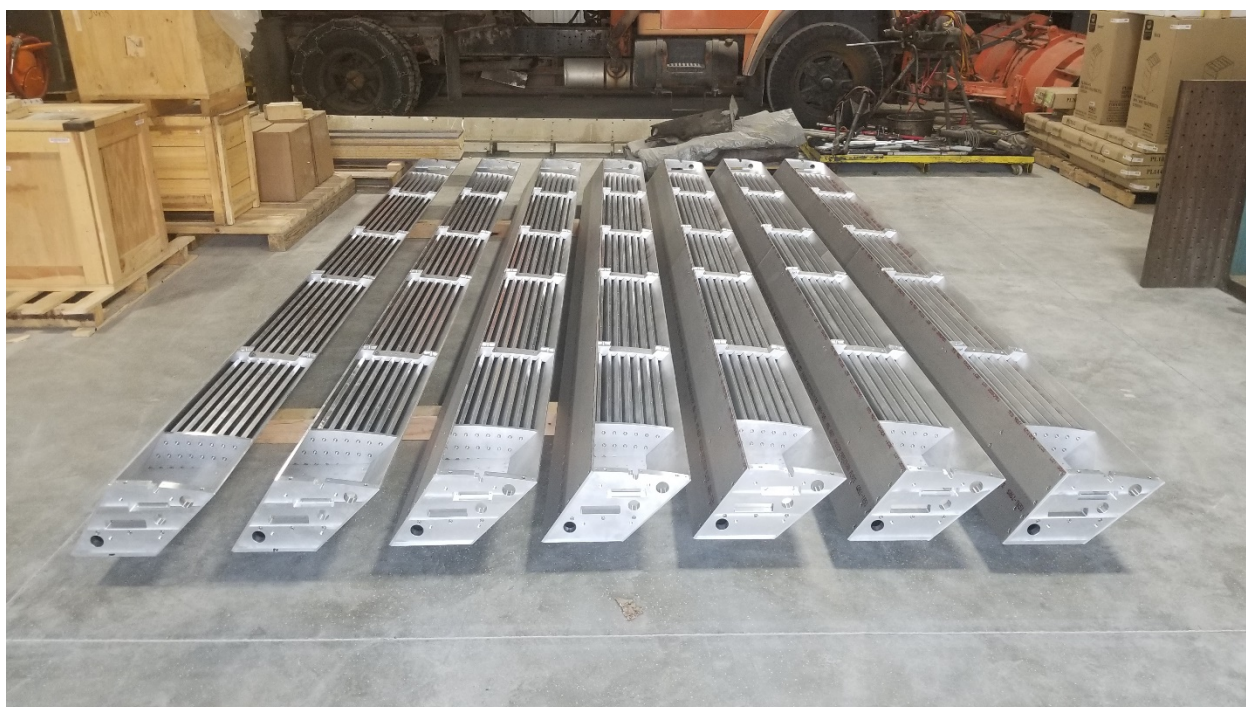
Figure 9: The first seven of eight completed inner HCAL sector in the assembly fixture at TSI in Ames, Iowa, being prepared for shipment.
