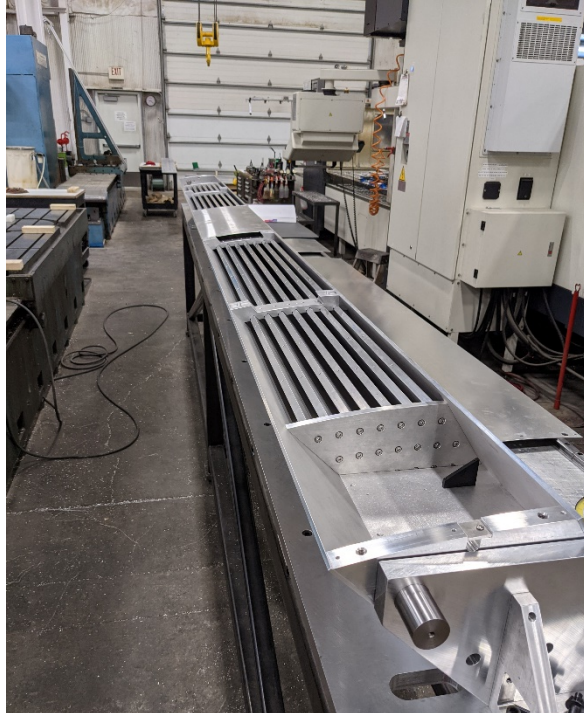
Figure 7: The first completed inner HCAL sector in the assembly fixture at a machine shop in Ames, Iowa. Only minor issues were identified during assembly and first article inspection, and the assembly of the remaining seven sectors for the first delivery to BNL later in June is underway.
