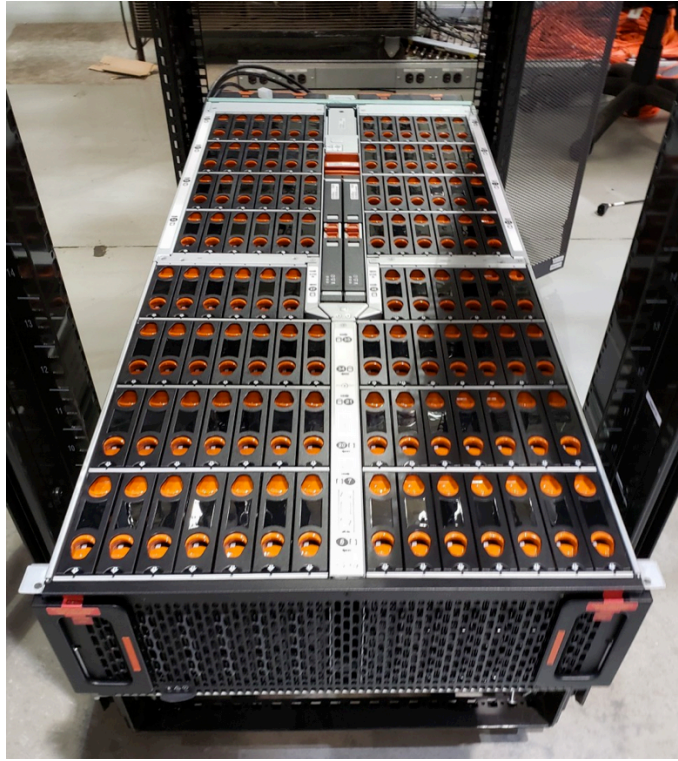
Figure 8: A picture of the disk enclosure with 102 14TB disks during setup.
