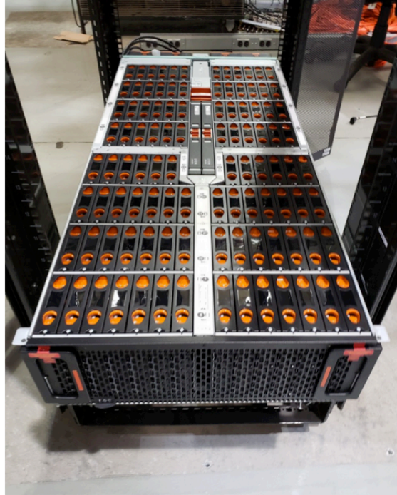
Figure 8: A picture of the disk enclosure with 102 14TB disks during setup.
