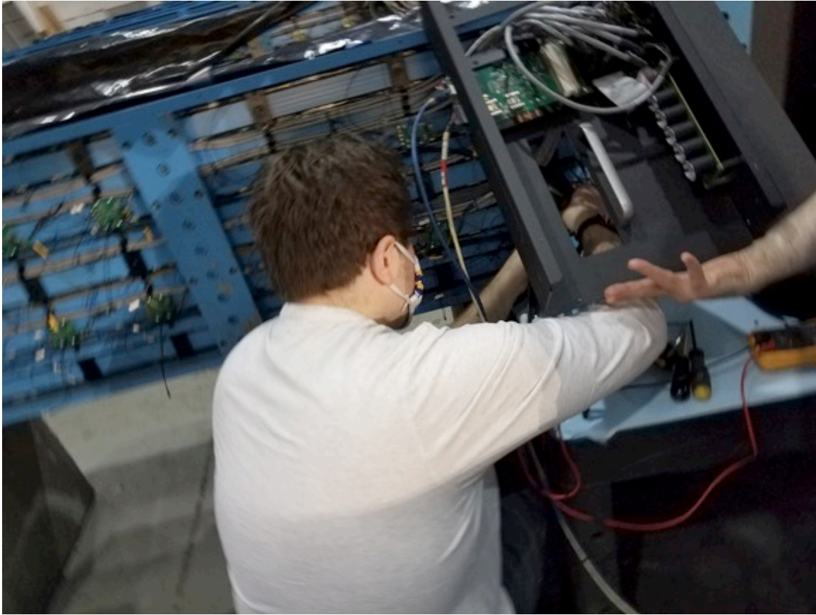
Figure 7: UC Boulder graduate student replaces a preamplifier on an outer HCal sector in the 912 factory.
