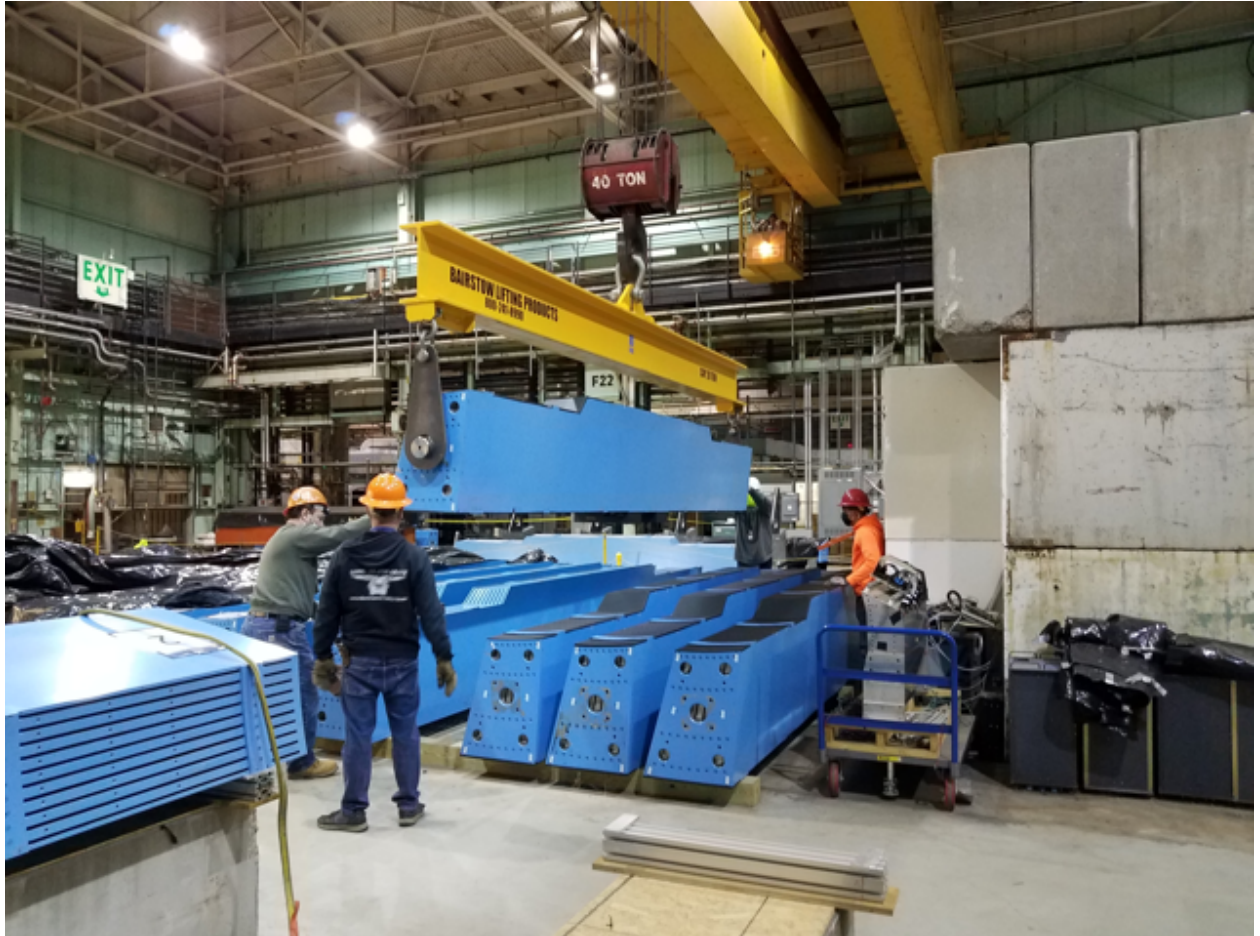
Figure 7: sPHENIX-BNL technicians along with BNL riggers, move completed OHCAL sectors into storage.
