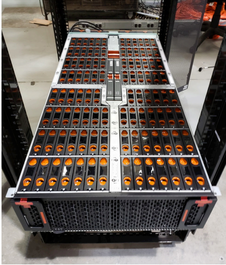
Figure 8: A picture of the disk enclosure with 102 14TB disks during setup.
