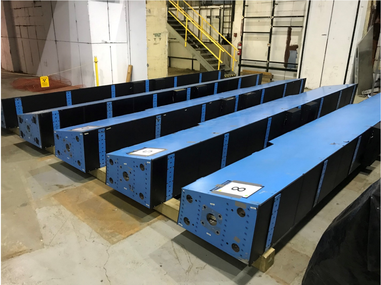
Figure 6: The 912 factory oHCAL storage area showing the first five fully completed pre-production sectors.
