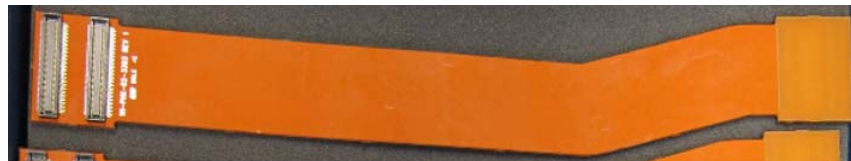
Figure E.12: The bus extender for FVTX.
