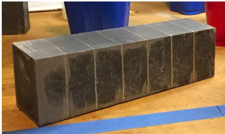
Figure 3.7: 2D projective block produced at Illinois.
