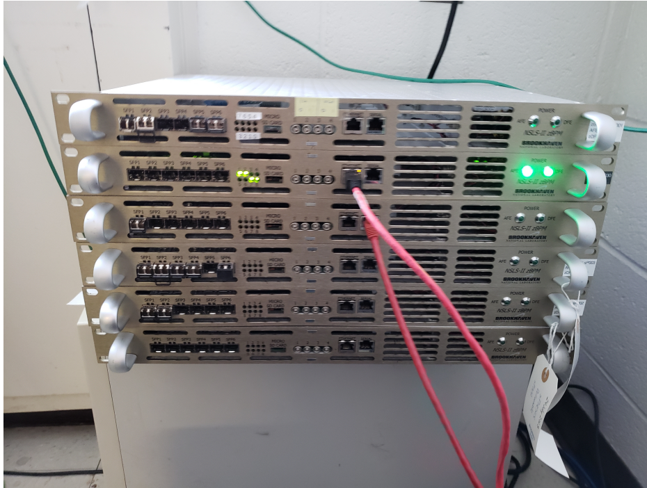
Figure 7.9: A picture of our candidate boards to run both the GL1 and the Timing System, depending on the installed firmware. We have 6 boards in hand that are used in various systems to implement the GL1 and timing system firmware.
