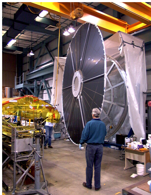
Figure 2.58: Photograph of the central membrane of the STAR TPC. The pattern of Aluminum strips is used to release electrons via laser flash as a calibration signal.
