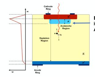
Electric Field: ~ 300 kV/cm in *Gain Layer* Adjustable Gain: ~2-100
