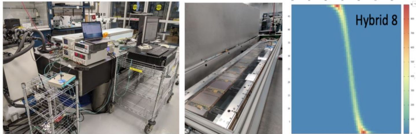
Figure 1: a) ATLAS ITk Strip Stave and FELIX readout at BNL. (b) ATLAS ITk Strip Stave. (c) ITk Strip Sensor s-curve calibration obtained using FELIX card.
