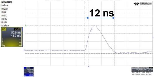
Amplifier with silicon detector fast enough to separate successive sources for eRHIC Linac Ring at 10 MHz
