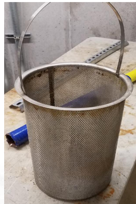
Sediments Collected in coarser strainer (now being primary in the system)
