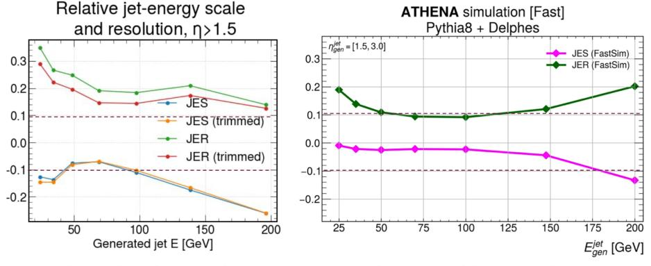
±10% lines indicated on vertical axes for comparison. Calorimeter model in fast simulation comes from YR, with ECAL (HCAL) constant resolution terms of 2% (10%) in the forward direction.
