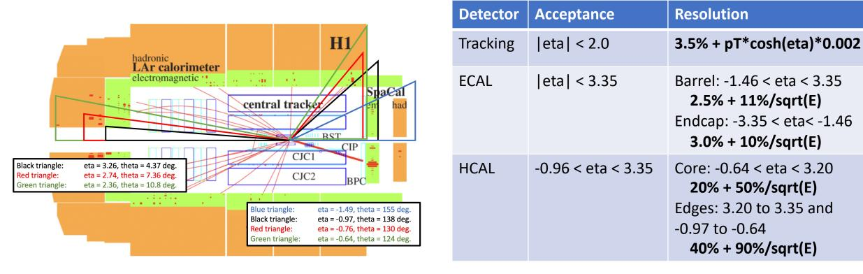
Resolutions based on NIM A 386 (1997) 310 with very rough adjustments from trial and error (not a systematic tuning yet).
