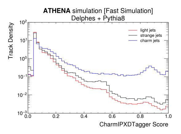
Based on the selection of jets using CharmIPXDTagger, we find the charm (light) jet efficiency to be 17% (0.86%). The expected yield of charm (light) jets in 100 fb<sup>-1</sup> is  $3.6 \times 10^3$  ( $7.3 \times 10^3$ ).
