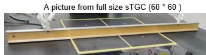
3100V Leakage current < 50 nA
