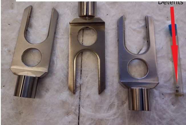
New forks with reduced width
