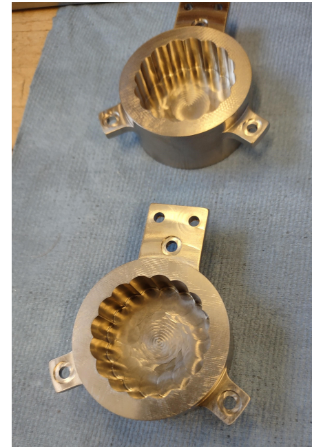
Cathode heater housing
