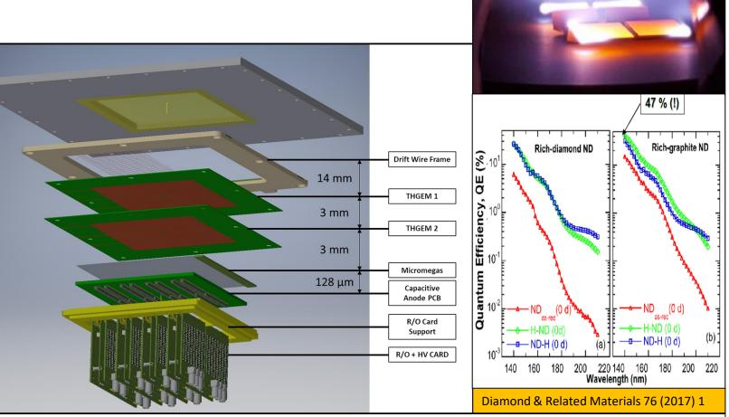
THGEM + MM hybrid Single Photon detector prototype with 3 X 3 mm<sup>2</sup> PADs with novel H-ND Photocathodes  $\rightarrow$  Ongoing R&D in INFN Trieste.
