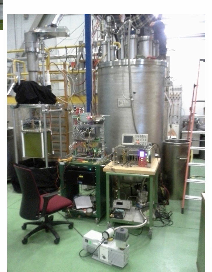
Monitoring the stress induced by shrinkage of CRP during a LN 2 bath test thanks to several strain gauges.
