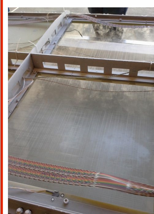
Checking wires tensioning.
