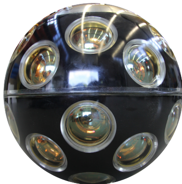
The KM3NeT Digital Optical Module.
