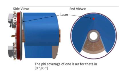
Static Distortions mapped (full 3D) by **line laser**. Magnetic field also mapped directly.
