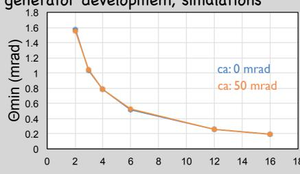
No practical impact of the beam crossing angle (ca) for the detection of the recoil nucleus.
