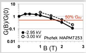
Photek MAPMT253 and Photonis XP85122-s-hice are viable candidates for  $B \le 2$  T and normal incidence. Relative orientation in the B-field is important.
